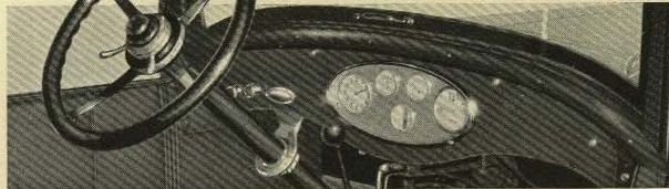
Handsome new instrument board showing instruments, grouped, under glass, on silver faced oval.
