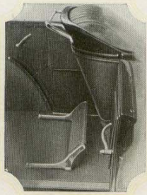
A nickel-plated hand and robe rail extends across width of seat. The carpet-covered foot rest is mounted on aluminum brackets.
