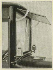
Completeness of Closed Cars is enhanced by one-piece rain-proof windshield with glare-proof visor and windshield cleaner.
